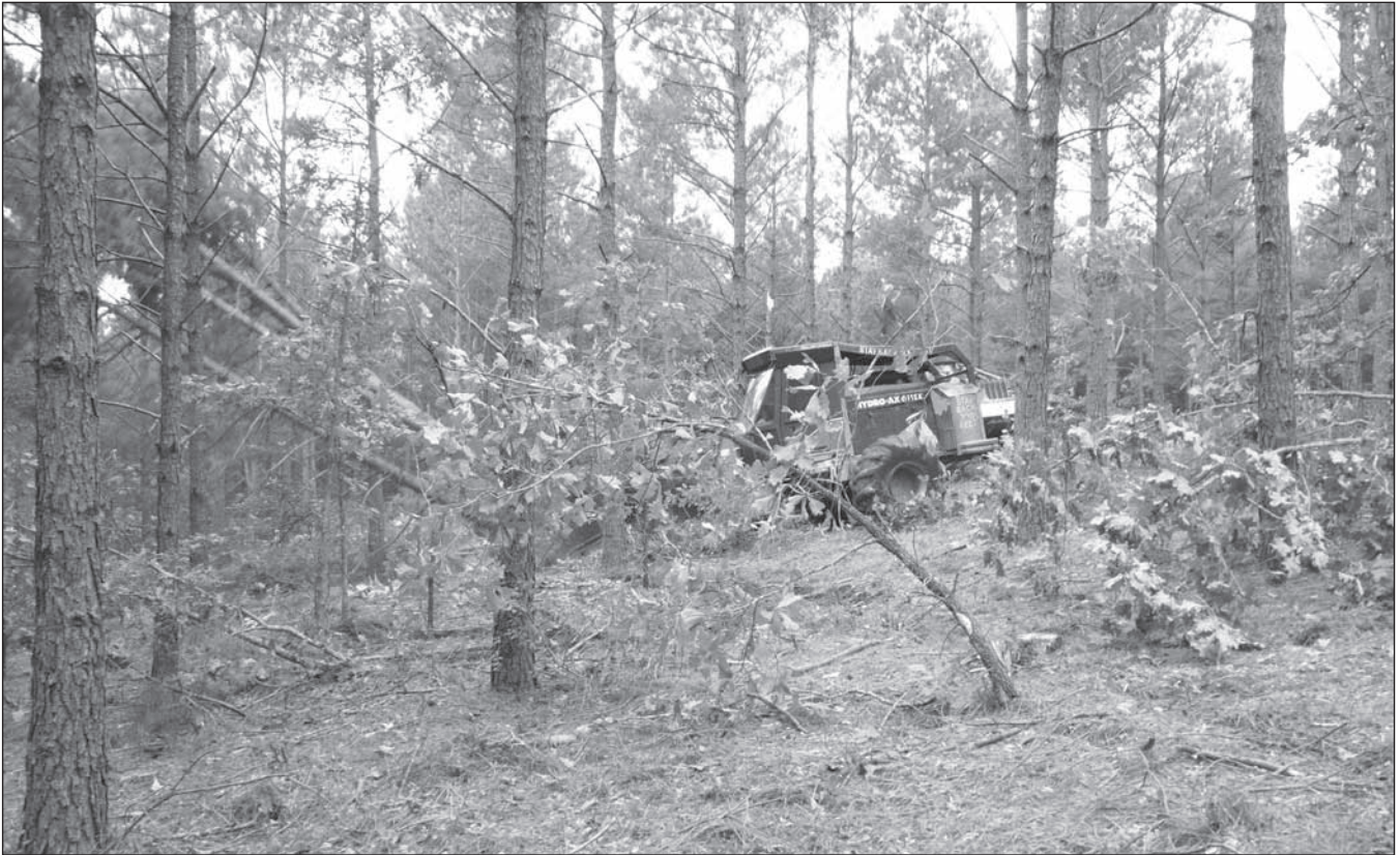
Feller buncher thinning in a 25-year old loblolly pine plantation. (photo by Tony Johnson)
